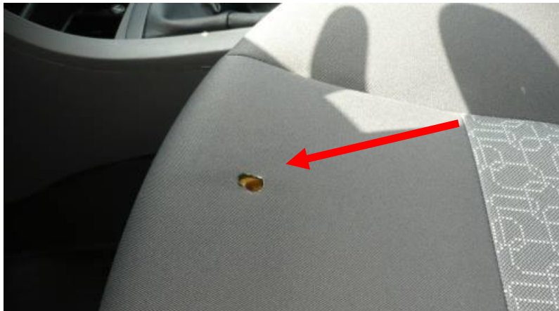
Seat trim damaged by cigarette burn, which may also occur on the back seats.
